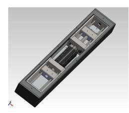
controls and data acquisition systems can be inside the vehicle, making it safer than manually carried units. Third, the configuration of the shock cavity and the coupling with the magnetic linear motor provides higher frequency content with better repeatability than those obtained using sledge hammers, elastic or explosive sources.
