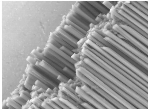
SEM image of carbon-carbon fiber composite
